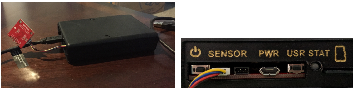
Figure 3.4: The sensor technology from cycle one including a front and side view. The red square is the environmental combo sensor. The LED labeled STAT turns green every time the readings from the sensor systems are written to the SD Card.
